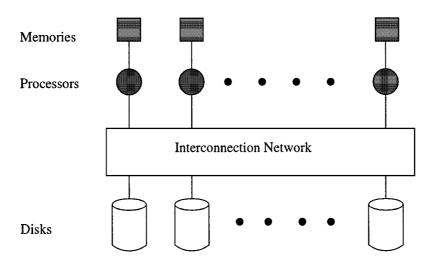
Figure 3. A schematic representation of shared-disk architectures.
