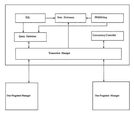
Figure 6. The PRISMA database architecture.
